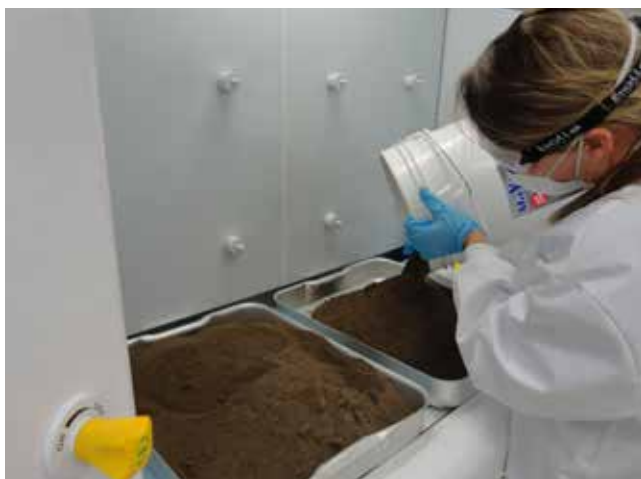
Preparing soils for RemBind treatment
