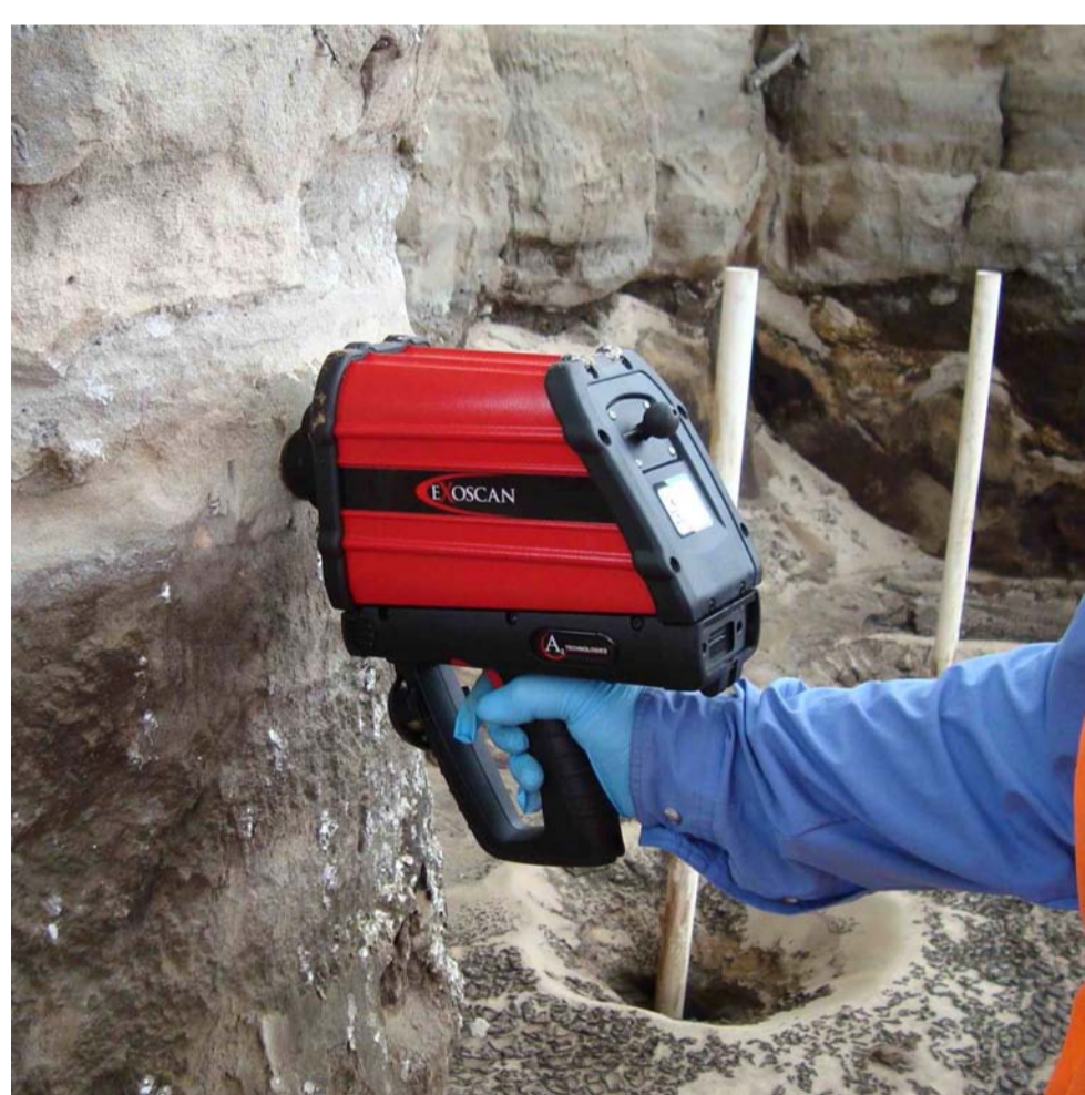
Figure 1: Field use of the hand-held MIR spectrometer, and an output display on the instrument.
